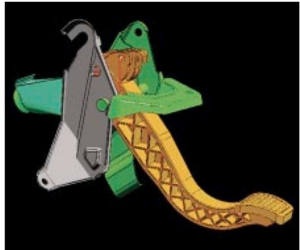
*Christian Müller, an ITESM-Toluca student, completed the first PACE project in Mexico, identifying a new material for the clutch pedal of the "S" car.*
